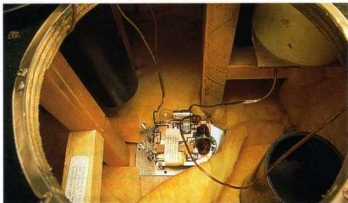
Contents under pressure: A special system of shimmed braces pushes out on the sides of the box. The result? Cleaner, deeper bass response.
